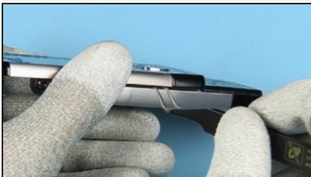
7. Shift open the slider. Carefully insert the tips of the angled tweezers into the recess as shown.
